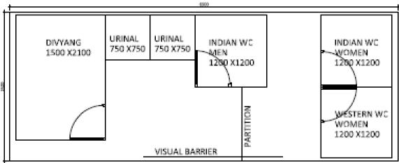
PLATFORM SIZE 6.5 M X 2.5M LEVEL +150MM APPROPRIATE RAMP TO BE PROVIDED
