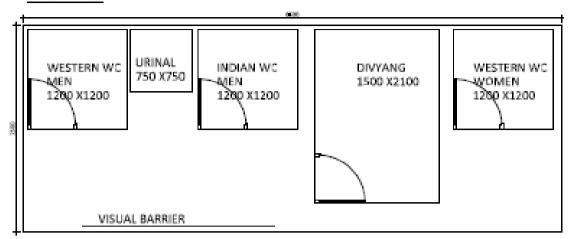
PLATFORM SIZE 6.5 M X 2.5M LEVEL +150MM APPROPRIATE RAMP TO BE PROVIDED
